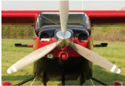
Passengers in its large cabin are protected by an extensive steel tube frame for maximum protection and safety. Both cabin and cowl skins are manufactured from lightweight carbon-fiber and advanced composites. However, the wing and tail are still made using traditional riveted aluminum skins for easy maintenance and repairability.
