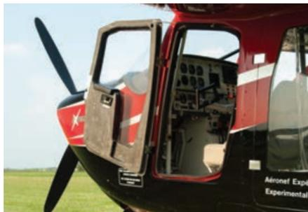
Safety is a very important part of the E-350 design including standard four-point harnesses for both pilot and co-pilot seats. Four doors that open 180 degrees, regardless of the flap setting come equipped with simple latch mechanisms for quick and easy egress of all passengers.
